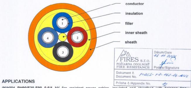
(N)HXH PH90/E30-E90 0,6/1 kV fire resistant power cables, insulated and sheathed with halogen free compounds, are intended for power supply to fire protection equipment which is to operate in fire conditions (e.g. water pumps in fire extinguishing systems, smoke removing fans).
