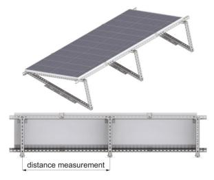
2. Measure the distance between the axes of the triangular structures.
