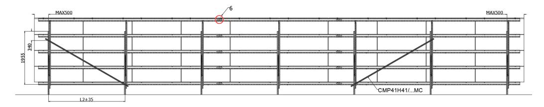
Fig. 2 View of the structure with bracing spacing No. 2
