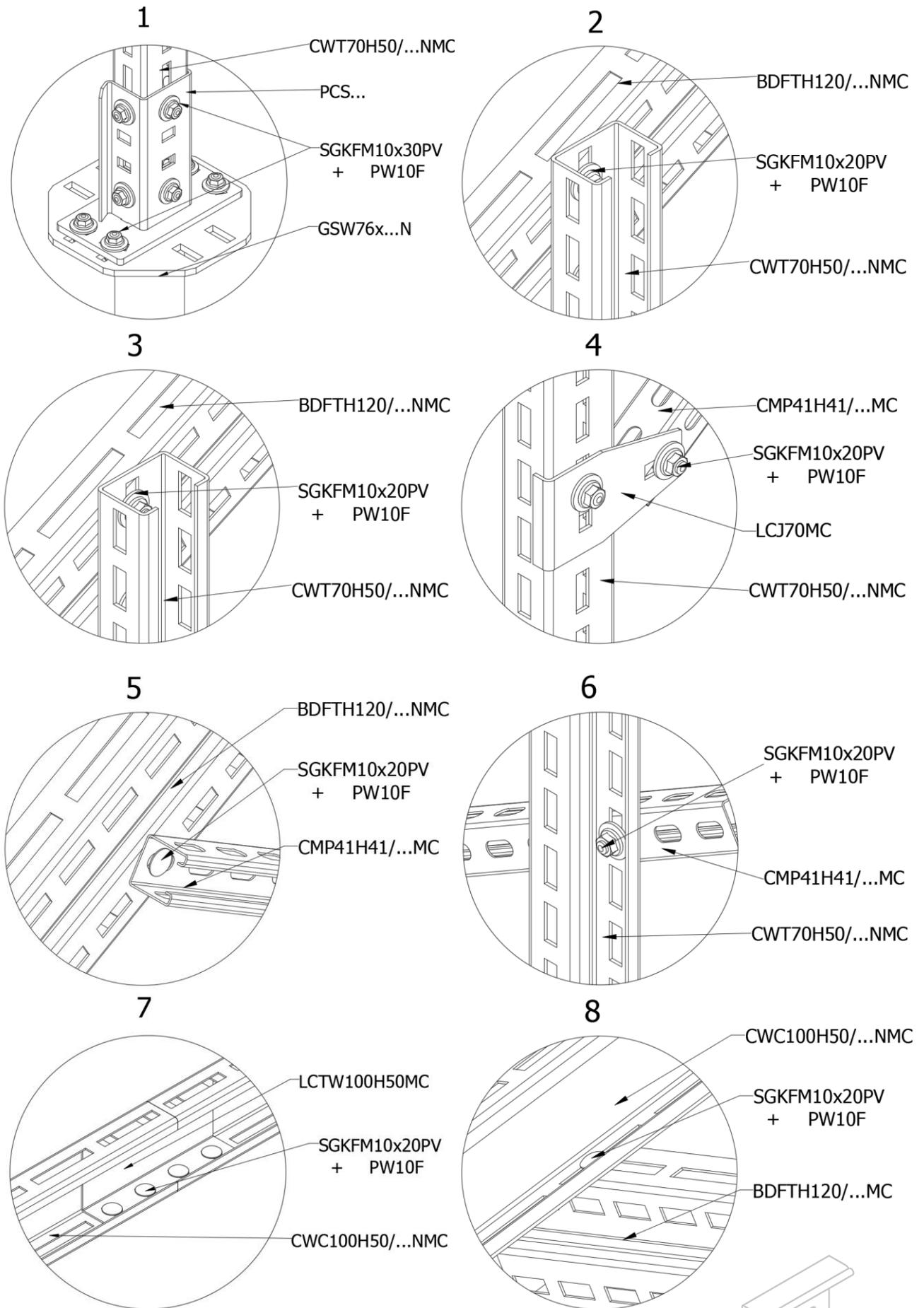
Fig. 3 Details of connecting the individual components
