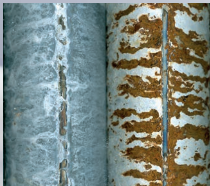
Magnelis® ZM120 welded, not re-protected
