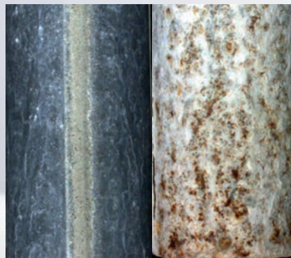
Magnelis® ZM310 welded and re-protected
